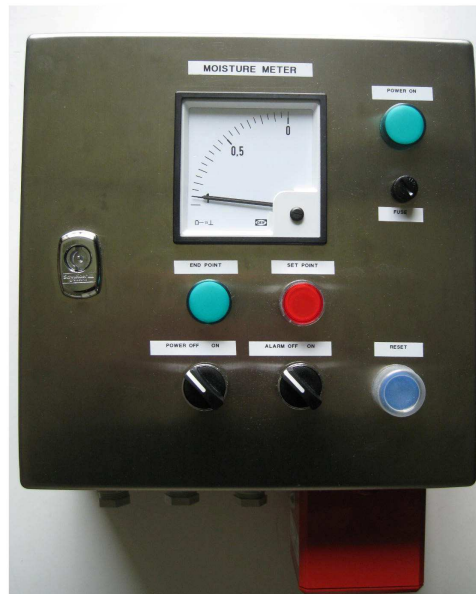
Moisture index meter with probe for automatic end-point control
